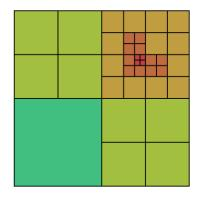
Schematic example of a refined grid Suárez Fernández et. al: arXiv:2205.04379v1
